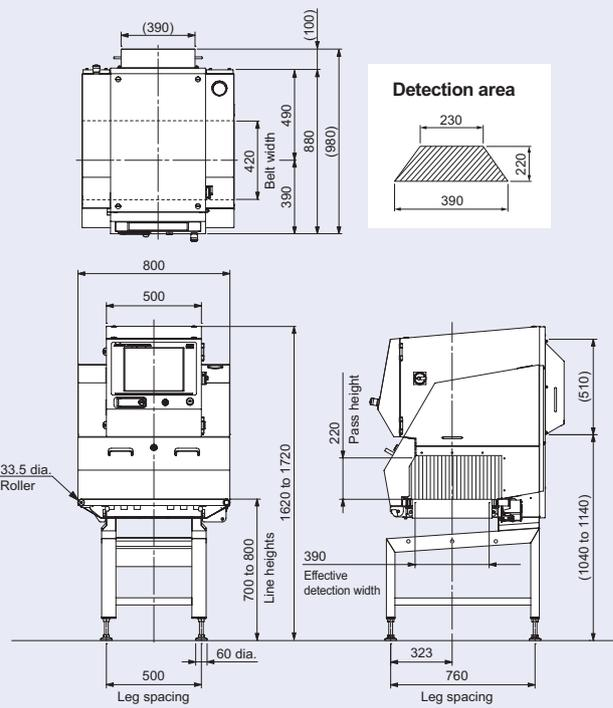
Dimensions in brackets are waterproof on the entire surface. Units: mm
